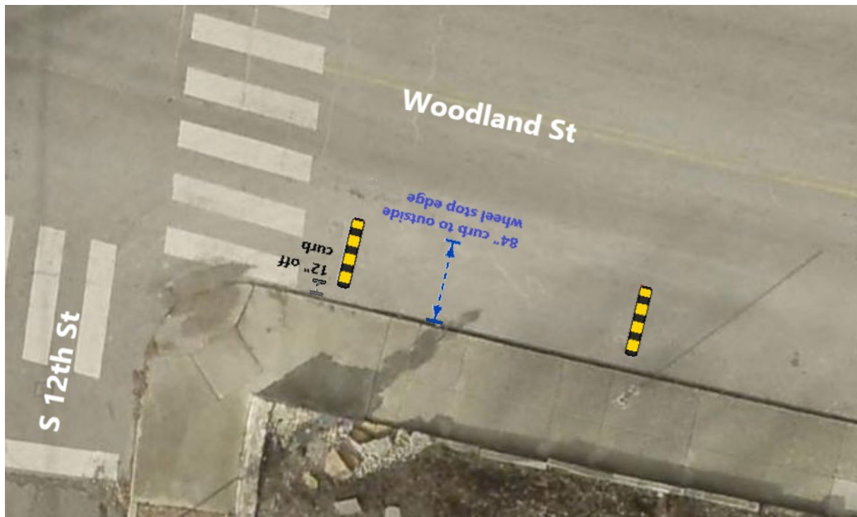
FORM B - SE corner of Woodland St & S 12 th St: Woodland St side
